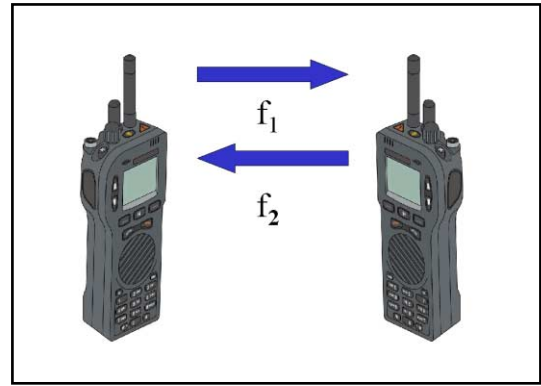
Figure 2.0 Two-way radio communication using duplex operation
