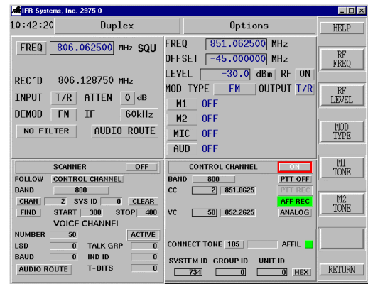
Figure 14.0 800 MHz Band Operation
